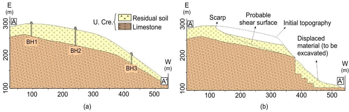
**Fig. 3.** A-A' cross-section before the production process in the quarry (a) and after the landslide (b)
