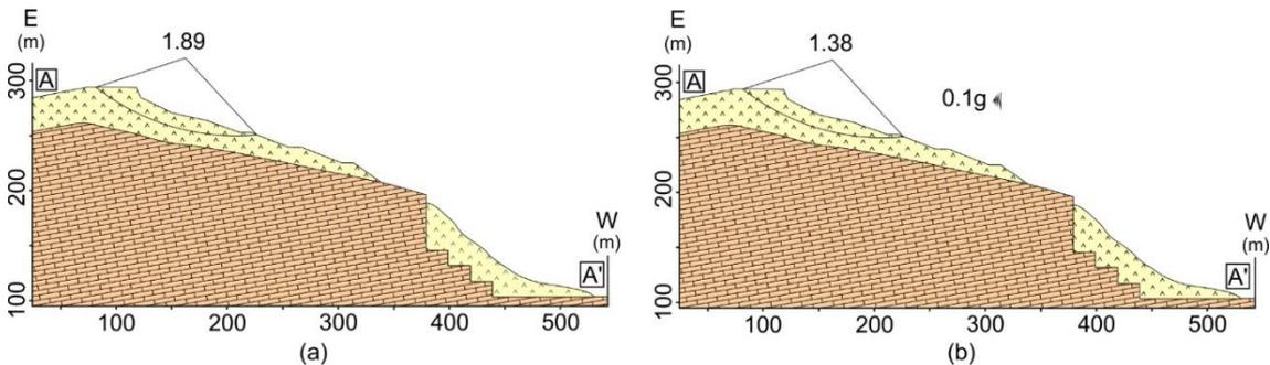
**Fig. 6.** Stability analyses with (a) and without (b) seismic effect for the new slope geometry
