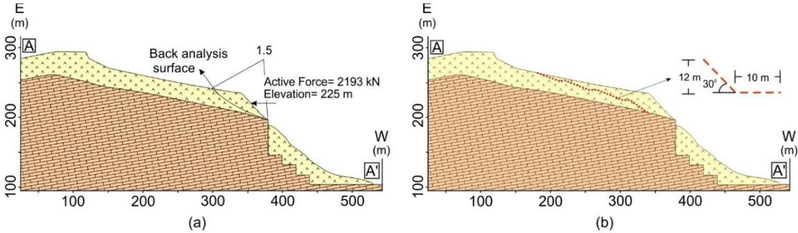
**Fig. 5.** Support back-analysis (a) and new slope design (b) for the slope
