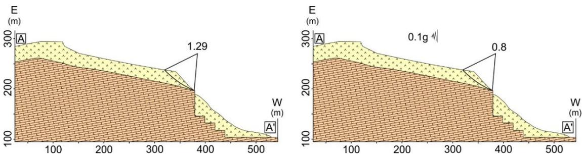
Fig. 4. Post-shear stability analyses with (a) and without (b) seismic effect along A-A' cross-section
