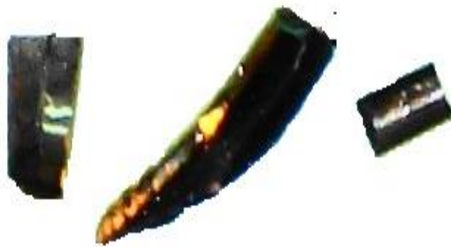
Fig. 1. General view of \text{Cu}_3\text{Fe}_{0.5}\text{Se}_2 single crystals ( \times 4 )
