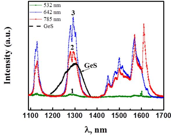
**Fig. 1.** PL spectra of pure GeS (solid line) and GeS:Nd at room temperature. (1-532 nm, 2-642 nm, 3-785 nm laser)
