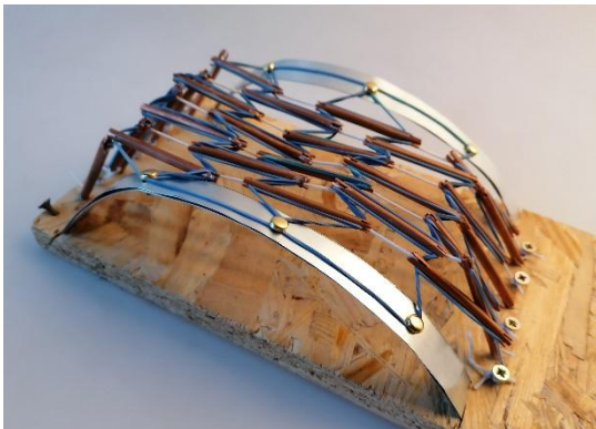
Figure 15. Physical model of the vault representing the tensile strength of the structure
