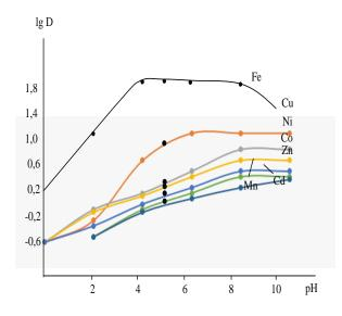
Figure 5. The dependence of the distribution coefficients of the elements on the concentration of hydrogen ions for the reagent  $R_5$
