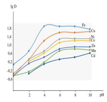
Figure 2. The dependence of the distribution coefficients of the elements on the concentration of hydrogen ions for the reagent  $R_5(1)$ ,  $R_4(2)$ ,  $R_3(3)$ ,  $R_2(4)$ ,  $R_1(5)$
