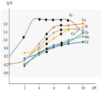
Figure 1. The dependence of the distribution coefficients of the elements on the concentration of hydrogen ions for the reagent  $R_2$
