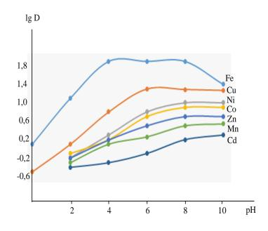
Figure 4. The dependence of the distribution coefficients of the elements on the concentration of hydrogen ions for the reagent  $R_5(1)$ ,  $R_4(2)$ ,  $R_3(3)$ ,  $R_2(4)$ ,  $R_1(5)$
