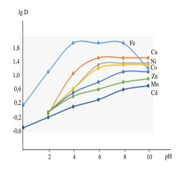
Figure 3. The dependence of the distribution coefficients of the elements on the concentration of hydrogen ions for the reagent  $R_5(1)$ ,  $R_4(2)$ ,  $R_3(3)$ ,  $R_2(4)$ ,  $R_1(5)$
